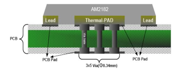
Figure 7 Recommended Via holes placement
